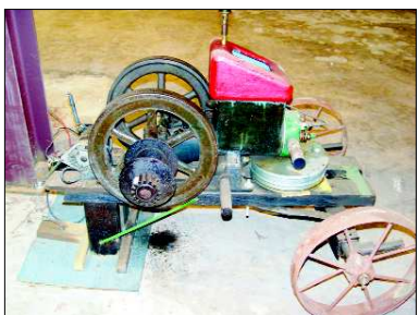
The Swansons replaced this old pecan cracker with a new, high-speed model. The old model cracked 50 nuts per minute compared to the new machine's 500 nuts per minute.
